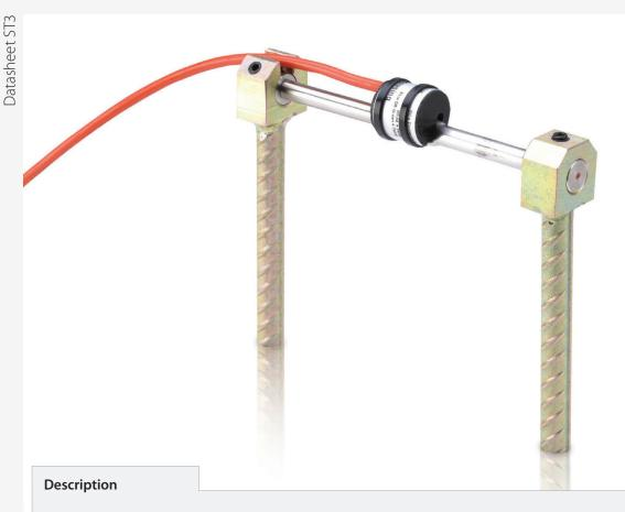
The Concrete Surface Mount Strain Gauge measures strain in concrete members. It consists of a coil assembly, Vibrating Wire element and two groutable anchors to embed the unit in the concrete structure to be monitored.
